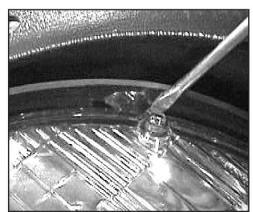
TAKE CARE WHEN REMOVING THE LAMPS. TO REMOVE THEM, PRY AT THE THUMB NAILS WITH A SMALL SCREWDRIVER. PRY ALL THREE A LITTLE AT A TIME UNTIL THE LAMP IS FREE. IF YOU HAVE QUESTIONS CALL US
