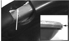
ON THE SNAKE EYE OR BLUE DOT LAMPS, THE THUMB NAILS SNAP INTO GAP BETWEEN THE GLASS AND THE HOUSING, NOT OVER THE GLASS. SEE PHOTO ABOVE.
